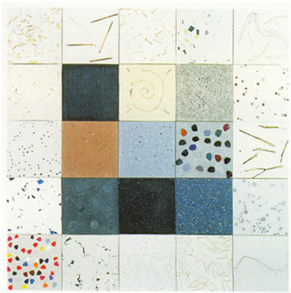
● Bottom, left: “Syn-decrete”, a cement-based composite tile with natural minerals and a variety of post-consumer scrap materials patented by Syndesis. Right: two projects by Franklin D. Israel: the front of the Kaplan House, Malibu, 1991 (above); detail of the pool living in the Larry-Newman Pavilion, Hancock Park, 1988 (below).
